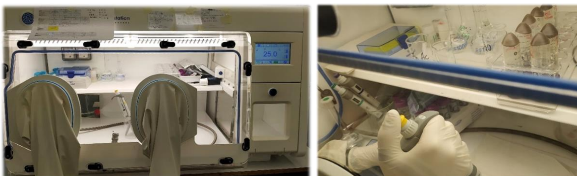
A glove box where work under no oxygen environment is guaranteed and the samples could be prepared for analyses.
