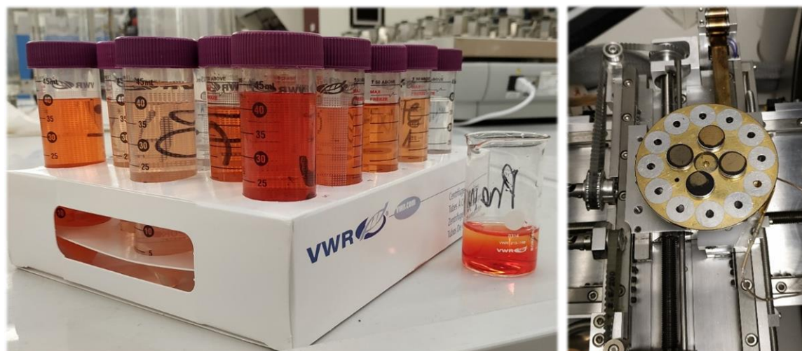
Liquid samples with different concentrations of Fe (left) and solid samples for STEM/EDS analysis (right).
